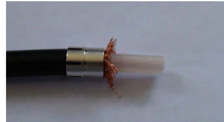
Fan out braid to allow collet fitting
