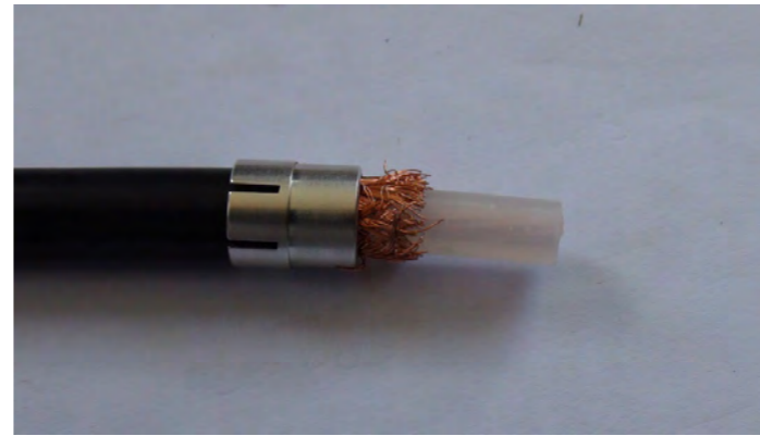
Slide on clamping ring
