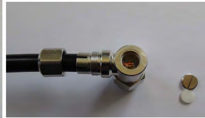
Fit connector body & solder
