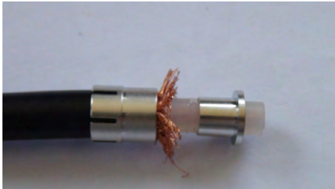
Slide Collet over inner dielectric
