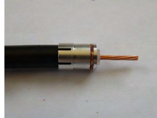
Trim Braid around collet Cut dielectric 1 mm from end
