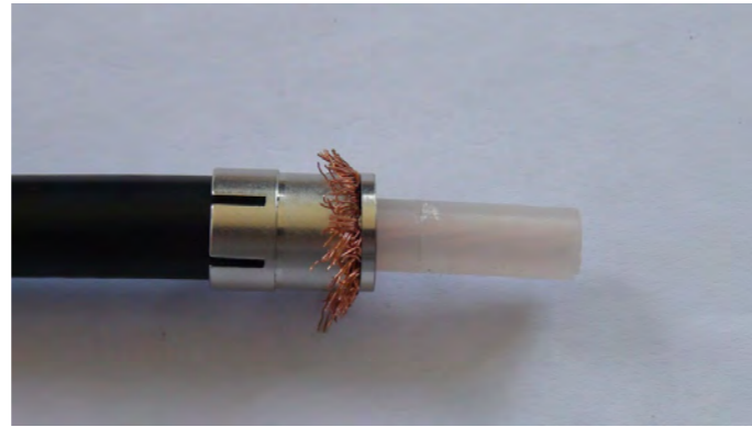
Press Collet firmly into braid
